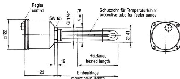
For pressure reservoirs made of refined steel or enamelled steel and anode screw-in type heaters ERCTBi will be used. In this finish the tubular heaters are mount galvanic isolated from gland G 1 1/2". Thereby, the protection current is prevented by the tubular heaters and the cathodic corrosion protection of the container barrier remains.
